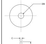
The use of snubbing washers is recommended to ensure proper static and dynamic loading of the isolator and retention of suspended equipment under severe shock environments.
