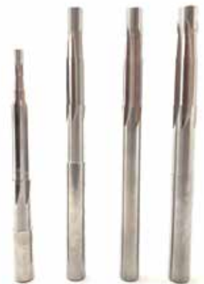
Chamber reamers produced by West Ohio Tool.
