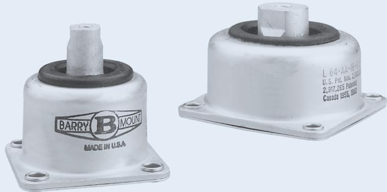
Barry L-Mounts increase equipment reliability and extend component life by providing isolation for frequencies as low as 10 Hertz and exhibiting low transmissibility at resonance (below 2.5) with 0.060" double amplitude vibratory input.
