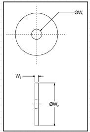
The use of snubbing washers is required to ensure proper static and dynamic loading of the isolator and retention of suspended equipment under severe shock environments.
