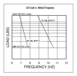
Figure 2 – L64 Load vs. Natural Frequency Comparison
