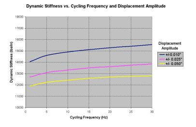
Figure 1 - Effect of strain (amplitude) and strain rate (frequency) on dynamic stiffness
