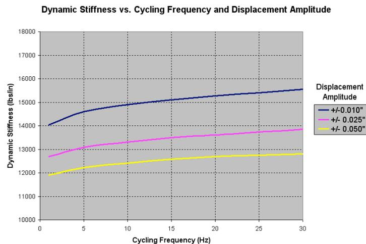
Figure 1 – Effect of strain (amplitude) and strain rate (frequency) on dynamic stiffness
